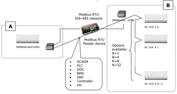
A Integration of single AC unit from independent XYE bus using INMBSACA001I000 interface
