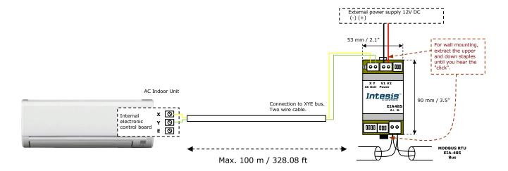
Figure 2.1 INMBSACA001I000 connection diagram
